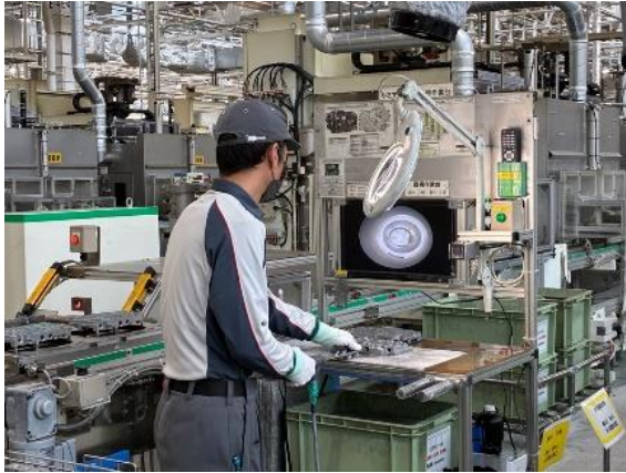
conventional visual inspection
