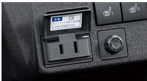
Accessory outlet (AC 100V・1500W/1 unit/with emergency power supply system)
