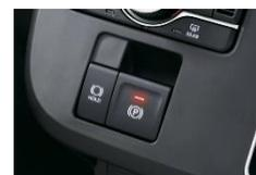
Electric parking brake & automatic brake hold function
