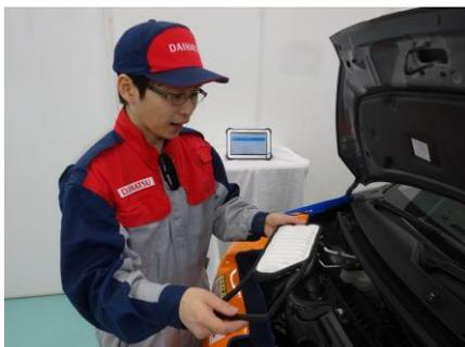
A mechanic inspects an air cleaner element. The results of the inspection are spoken into the microphone attached to his chest, and then automatically entered into the tablet terminal shown in the background of the photograph.
