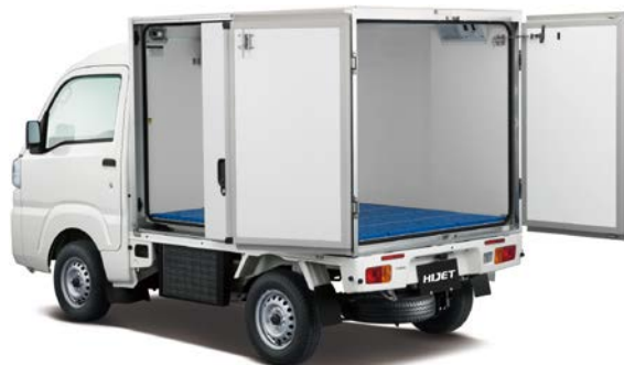
The Hijet Truck, a colored aluminum medium-temperature refrigerator car
