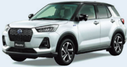
The e-SMART HYBRID system, used on the HEV Rocky, adopts a series structure in which an engine generates electricity to drive a motor.
