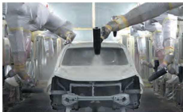
Deploying innovative technologies— Dry booths for painting processes
