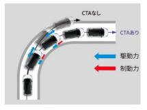
Schematic diagram of CTA in action
