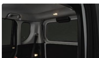
Luggage room lamps (deck right side and ceiling)
